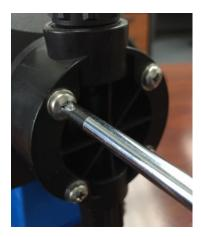
3. Remove the diaphragm. Pay attention to the brass shim washers behind the diaphragm and make sure the same numbers of shims are used during re-assembly.
